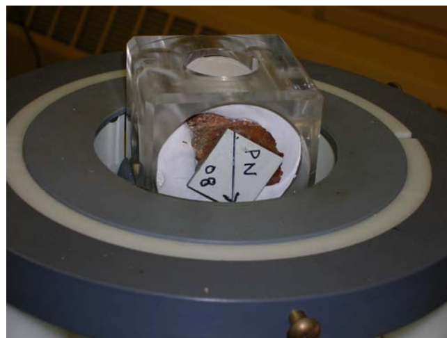
Figure 4. A typical sample being lowered into the cylindrical magnetic shield of the Molspin spinner magnetometer. The plastic square measures 2×2cm.
