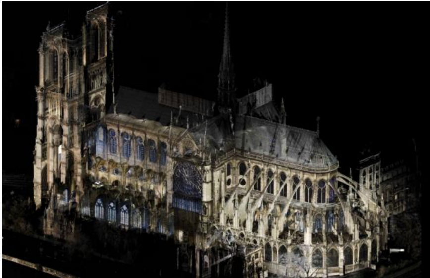
Figura 60: Escaneo digital de la Catedral de Notre Dame, París. por Andrew Tallon. Fuente: Jee, C. (2019). Recuperado de: This digital scan of Notre Dame offers hope for its restoration after the fire.
