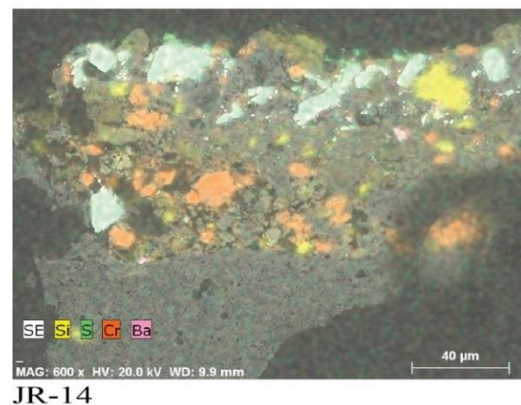
Figure 4.3.11. Distribution of Cr (orange) in three micro sample cross sections (JR10, JR12 and JR14)
