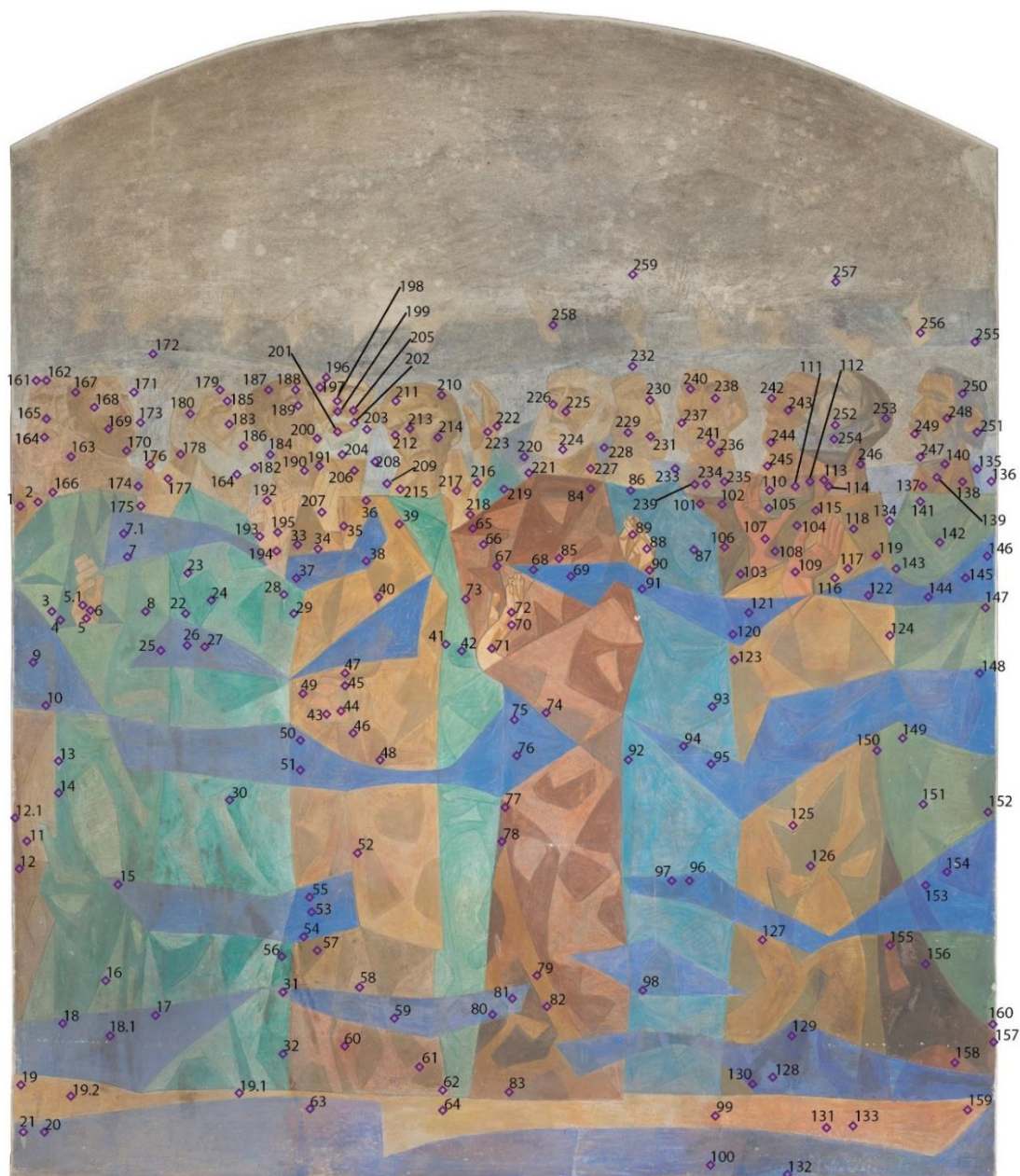
Figure 3.2.2 Map of the colorimetric measurements. Photo by Manuel Ribeiro 2018
