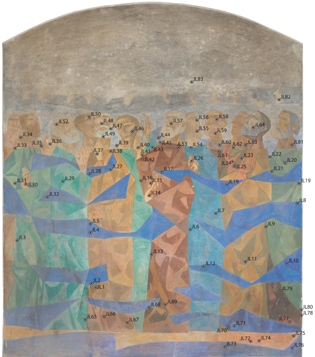
Figure 3.2.3 Map of EDXRF measurements of the paint layers. Photo by Manuel Ribeiro 2018
