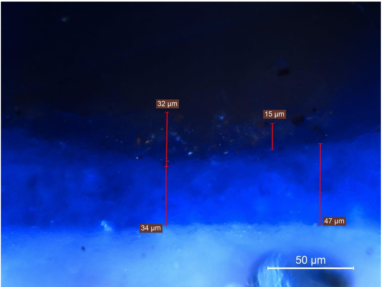
Figure 4.3.8. JR18 cross section. Layer of mixed Co and Ca (with presence of Red Ochre particles). Above on the left: EDS map showing distribution of Ca, Co, Si and Na; above on the right: EDS map showing presence of iron-rich particles (marked with yellow circles); below: OM picture of the cross-section with layer thickness indication.
