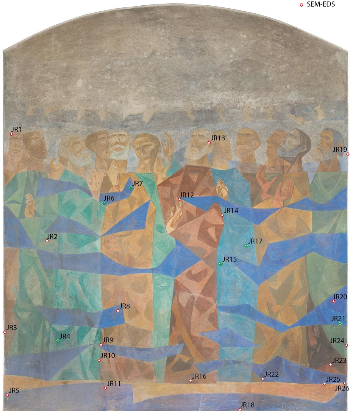
Figure 3.2.4. Map of the samples extracted for laboratory analysis. Green: powder samples for \mu -FT-IR and \mu -Raman examination; red: cross-sections for OM and SEM-EDS examination. In areas marked JR2, 14 and 25 both powder samples and cross-sections were extracted. Photo by Manuel Ribeiro 2018
