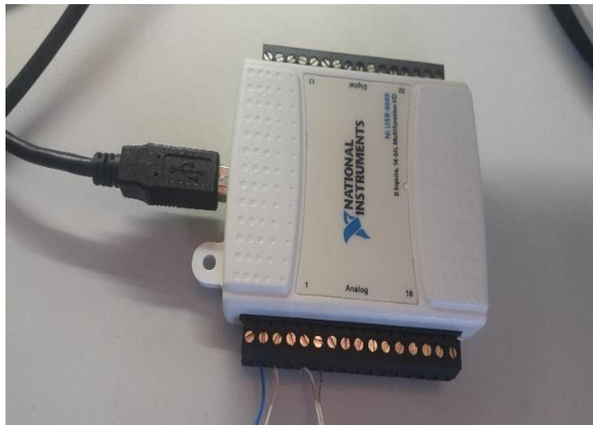
Figure 2.33 NI USB-6009 DAQ.
