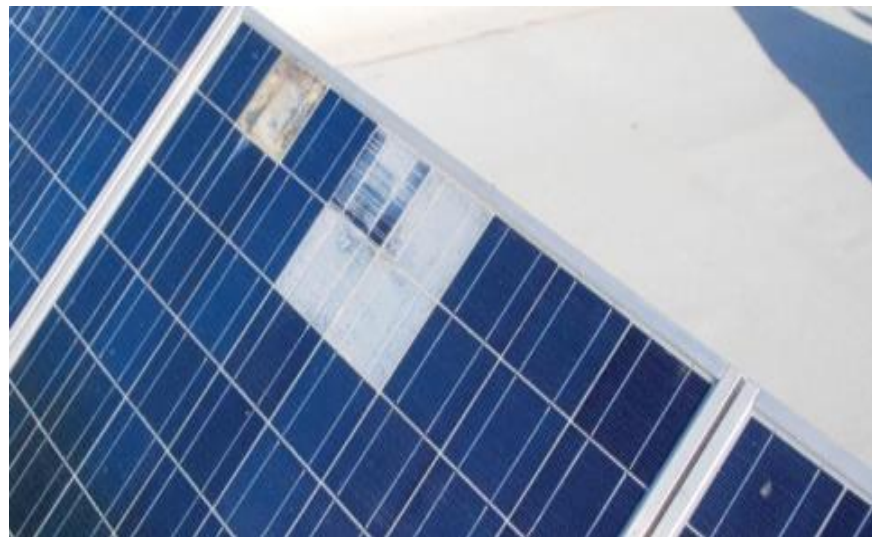
Figure 2.30 Physical damage as time-independent obstacles.
