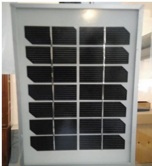
Figure 2.37 Monocrystalline silicon PV panel.
