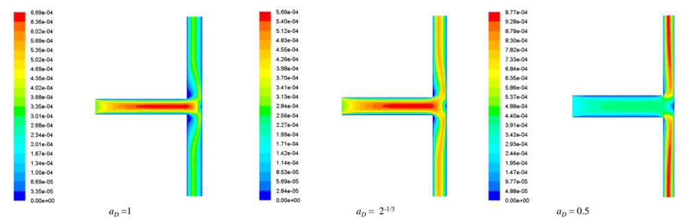
Figure 3. Velocity contours (middle plane) in a 3D T-structure ( $n = 1$ )
