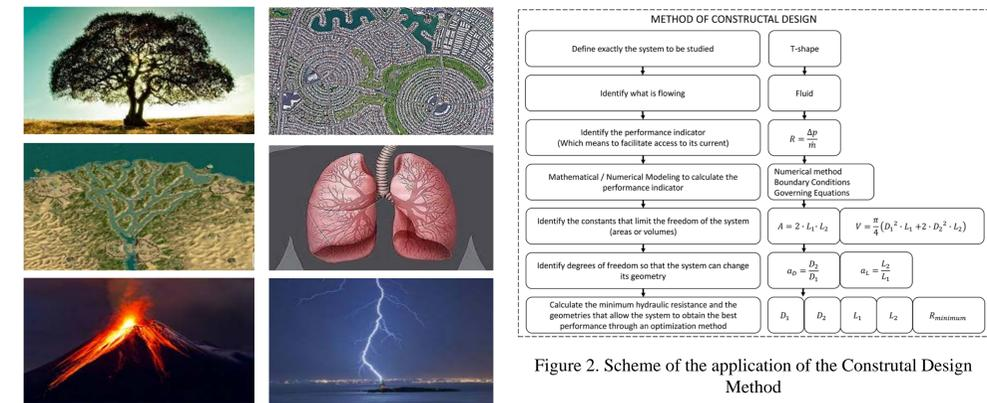
Figure 2. Scheme of the application of the Constructral Design Method
