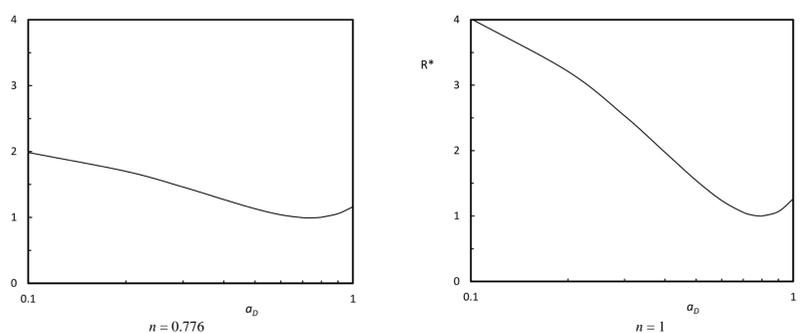
Figure 5. Dimensionless total flow resistance,  $R^*$ , of a T-flow structure.
