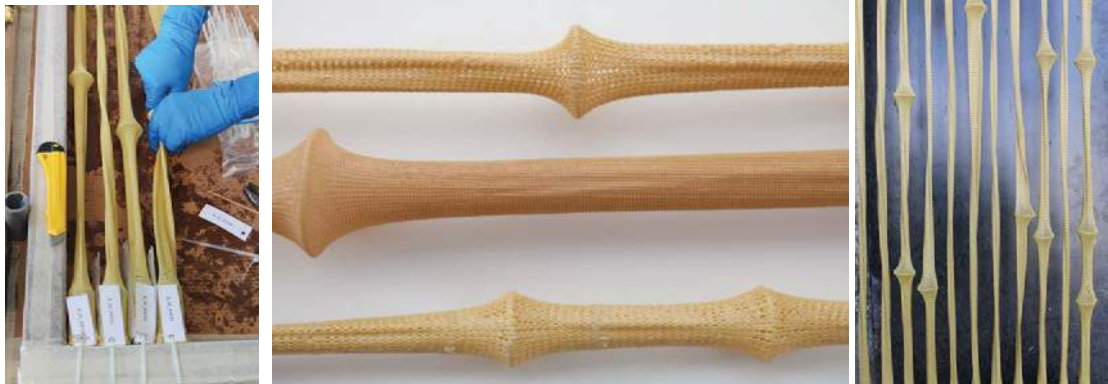
Figure 11. Fabrication process: shaping and curing not requiring moulds
