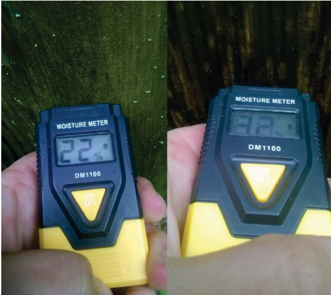
Figure 5. Moisture Content of Panels of Prototype Ray 2 with and without Algae in 8°C and 66% Relative Humidity after light April Rain (photo: Davidová 2017)
