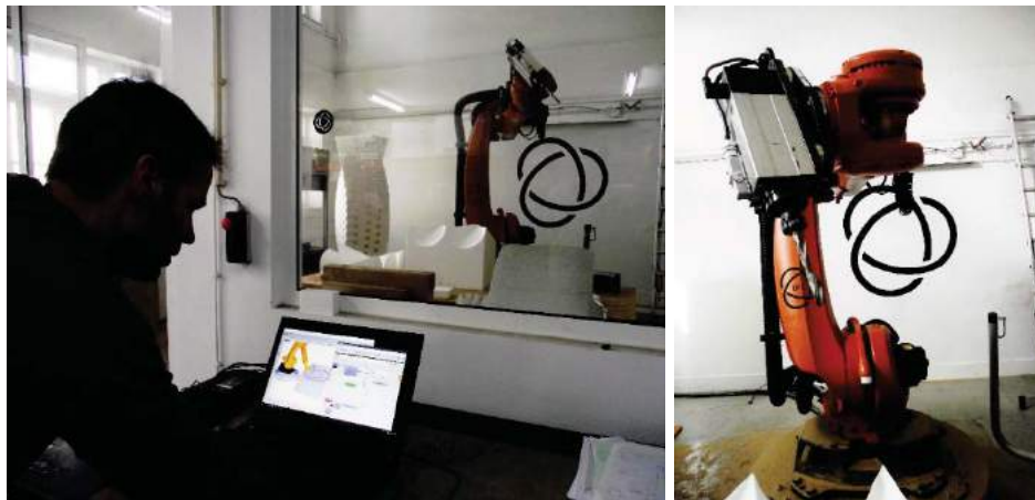
Figure 1. DFL space: image on the left - Professor José Pedro Sousa explaining how to maneuver the robotic arm; image on the right - The robotic arm with a tool prepared to mill.
