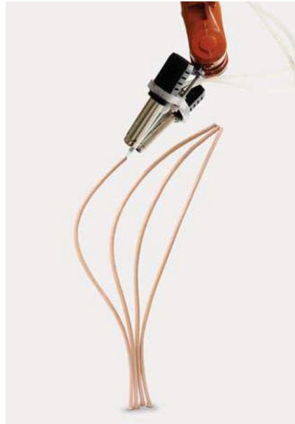
Figure 1. Plastic mix robotic extrusion creating gravity defying structures. Source: https://www.dezeen.com/2013/05/17/mataerial-3d-printer-by-petr-novikov-sasa-jokic-and-joris-laarman-studio/
