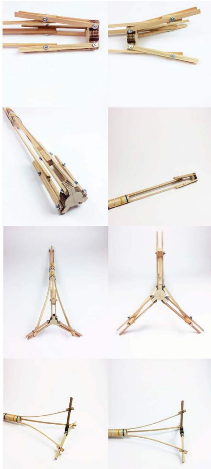
Figure 14. Physical prototype of a bistable mechanism using flexible wood strips to act as springs.
