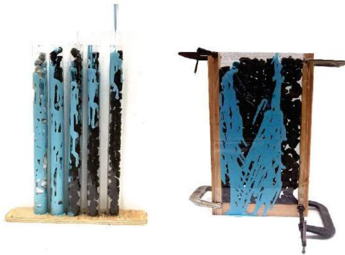
Figure 4. Sectional test measuring pour time to depth (left); sectional test measuring pour behavior after tilting (right).
