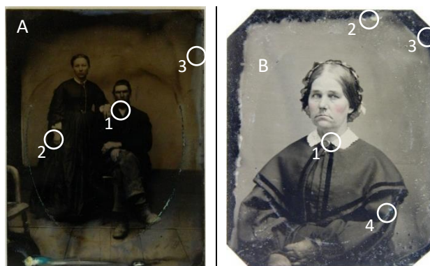
Figure 43: mapping of the areas analysed with SEM-EDS on tintypes A and B.
