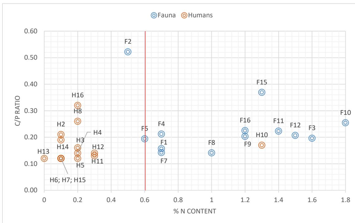
**Figure 22** Relative carbonate content by ATR-FTIR vs. % N content by EA.
