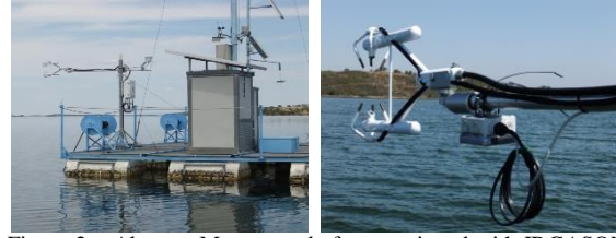
Figure 2 – Alqueva-Montante platform equipped with IRGASON instrument; Detail on sonic anemometer, gas analyser and accelerometer.
