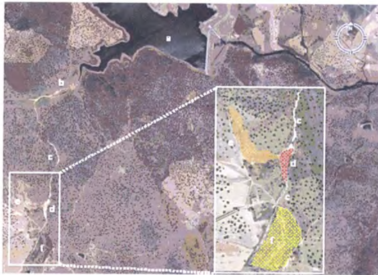
FIG. 1. Tinoca mine area. (a) Abrilongo River. dam; (b) Caga-no-ninho stream; (c) Mine stream; (d) abandoned mine sedimentation dam; (e) mine-waste deposit; (f) mine wastes encapsulated by a geomembrane and vegetation cover (photo: GoogleEarth)
