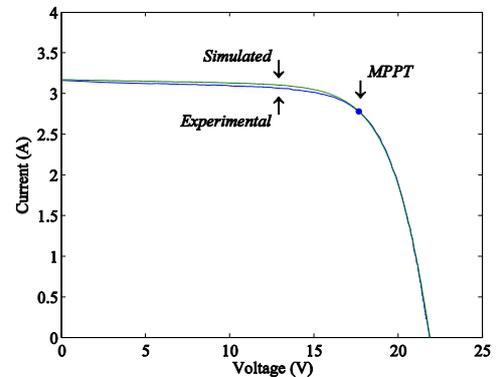
Fig. 1. I-V simulated and experimental curves at STC.
