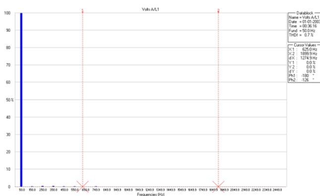
Fig. 2. Harmonic content of the output voltage.
