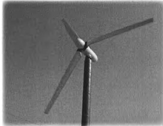
Figura 4.19: Turbina FD6.4-5000-16 (5000 W) (turbina B) <sup>[37]</sup>.
