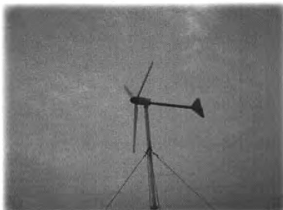
Figura 4.18: Turbina FD2.7-1000-10 (1000 W) (turbina A) <sup>[36]</sup>.
