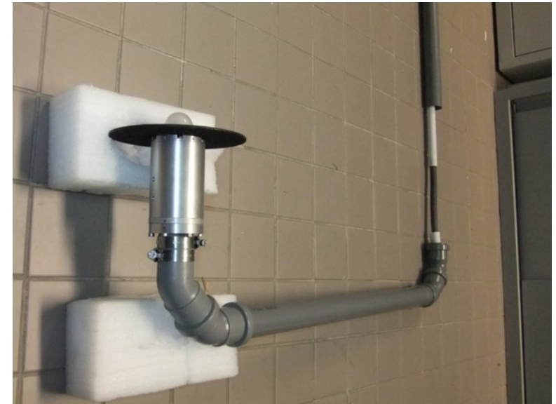
FieldSpec UV/VNIR da ASD coupled to an optical cable and a cosine receptor
