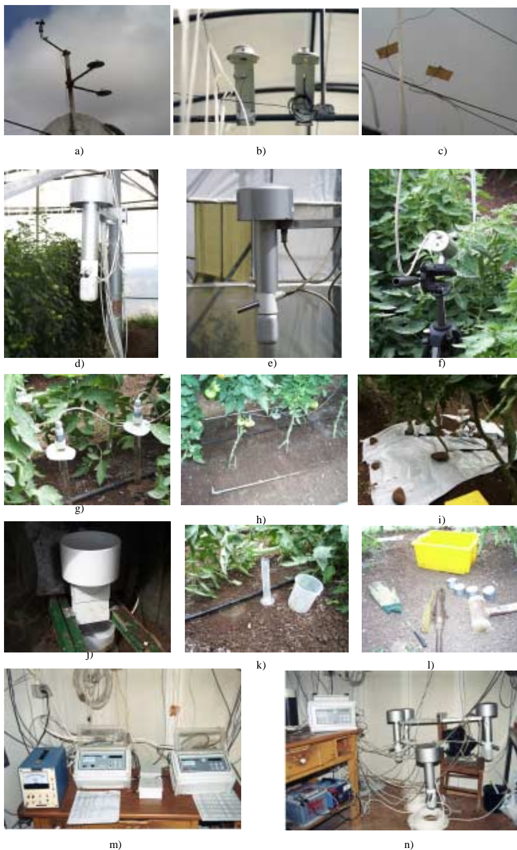
Figure 2.4 – Measuring and recording equipment used in the experiments: a) outside pyranometer, PAR radiation sensor and anemometer, b) inside pyranometer and PAR radiation sensor, c) cover thermocouples, d) inside psychrometer, e) outside psychrometer, f) infra red thermometer, g) tensiometers, h) lysimeter, i) plugged lysimeter, j) rain gauge, k) drip rate checking, l) soil sampling, m) data loggers, n) psychrometers checking
