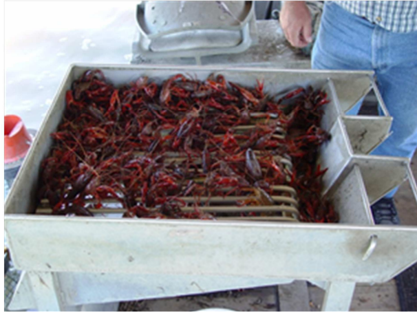
Figure 1. Representative example of one of several types of on-board graders designed to cull smaller sizes of crayfish from the catch in commercial aquaculture ponds. Photo by Ray McClain.
