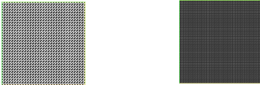
Figure 5.1: Structured meshes employed on square [0.25, 1.25] \times [0.5, 1.50] . The coarse mesh with 2048 elements (on the left) and the fine mesh with 8192 elements (on the right).
