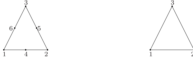
Figure 4.3: \mathbb{P}_2 - \mathbb{P}_1 elements: degrees of freedom for the velocity components (on the left) and for the pressure (on the right).
