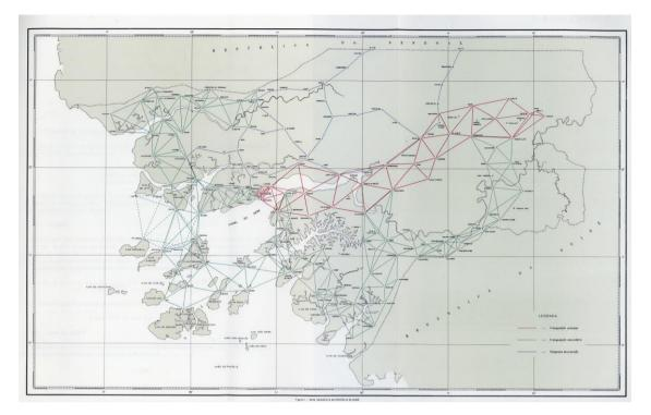
Figure 5 - Classical terrestrial triangulation network (IH, 1968).
