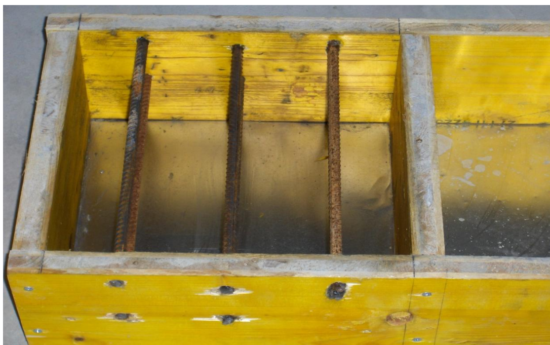
Figura 3.12 – Moldes de lajetas-molde individual
