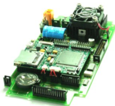
Figura 4.4 - Placa AMSRel.3 (Advanced Micro Stepping controller, Release 3).
