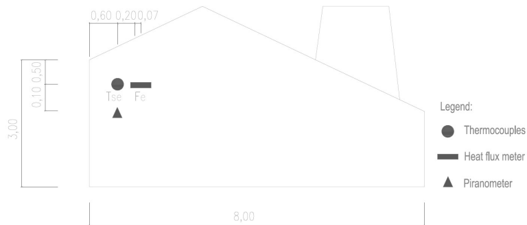
Fig.5. Sketch of the west façade with probes' location.
