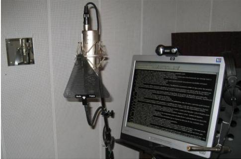
Figure 2: Control room. The display monitor on the right is a mirror of the recording booth monitor. The control station had two display monitors, one of them being mirrored inside the sound-proof room. These monitors were used to display the recording prompts under the control of the recording supervisor.
